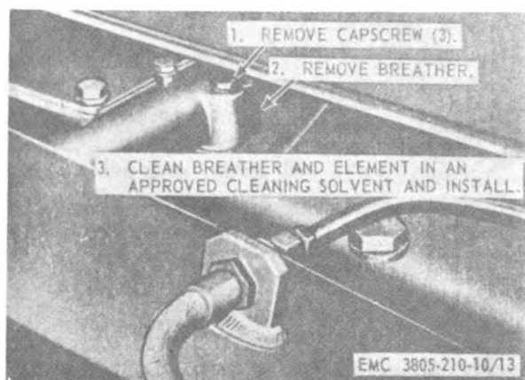
Figure 13. Transmission breather service.
